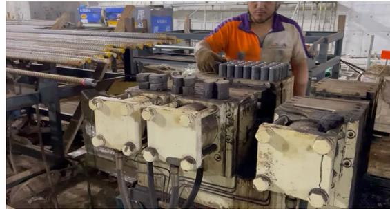
On-site Rebar Coupler Fabrication by **ONE-GO PROCESS**
