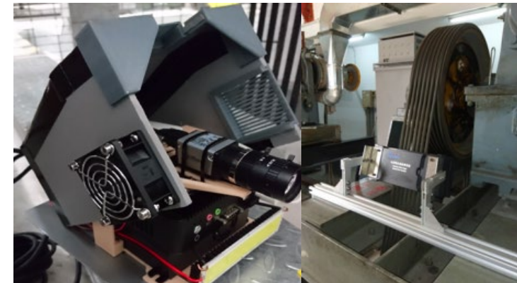
Real-time monitoring and defect detection, enables replacement only when health is poor e.g. visual and electromagnetic analysis of elevator rope.
