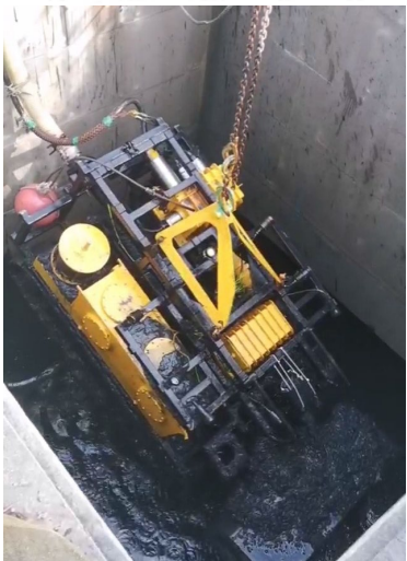
ROVPD with built-in CCTV HD camera and sonar loading down to water for desilting work
